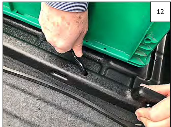
12 Hook your bungee cord through the new hole you created in Step 11.
