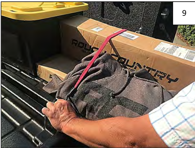
9 Use bungee cords (not provided) to secure items being stored in tray. Insert hooks through slots around perimeter of Bed Storage Tray. Criss Cross bungee cords to secure items.
