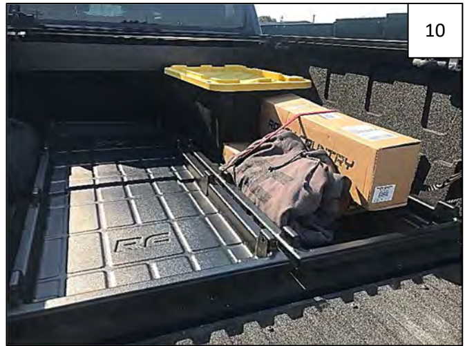
10 Slide tray back to close tail gate – tightened straps will keep tray from moving further into bed.
