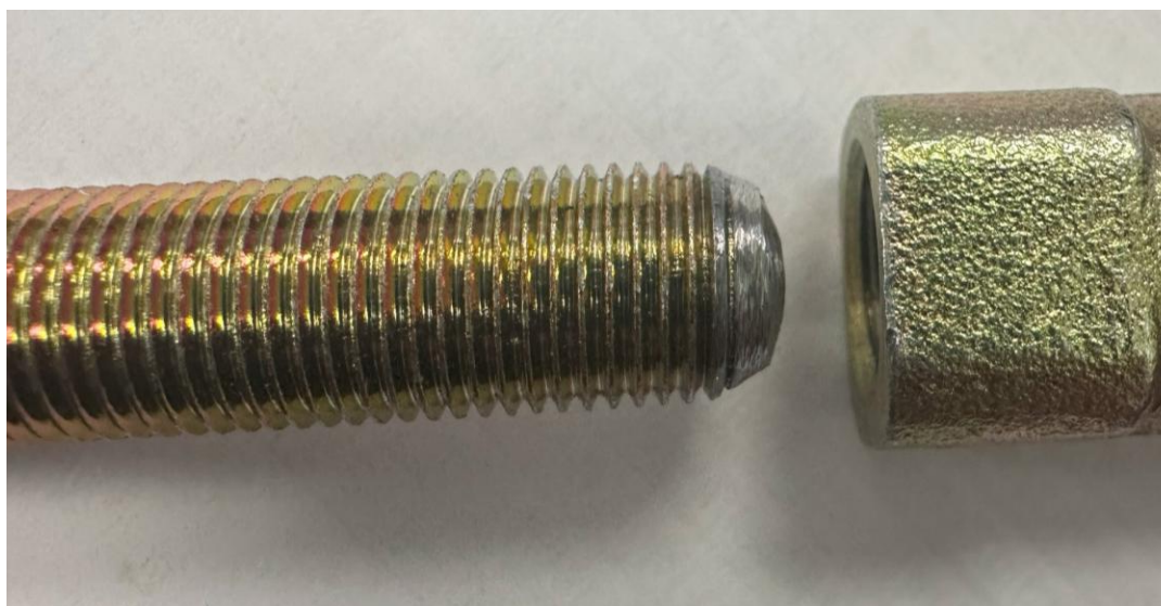
Figure 3: Beveled edge of sway bar rod with sway bar rod end
