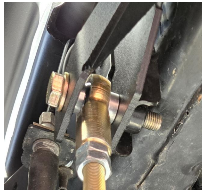
Figure 6: COR-5110200 with Heim Joint and "longer" bolt
