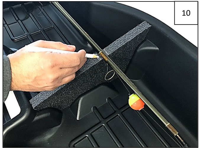
Use a marker or grease pencil to trace the width of the item on each Foam Divider. Remove item and trace the depth at which you would like the item to rest. NOTE: Cutouts should be fairly snug.
