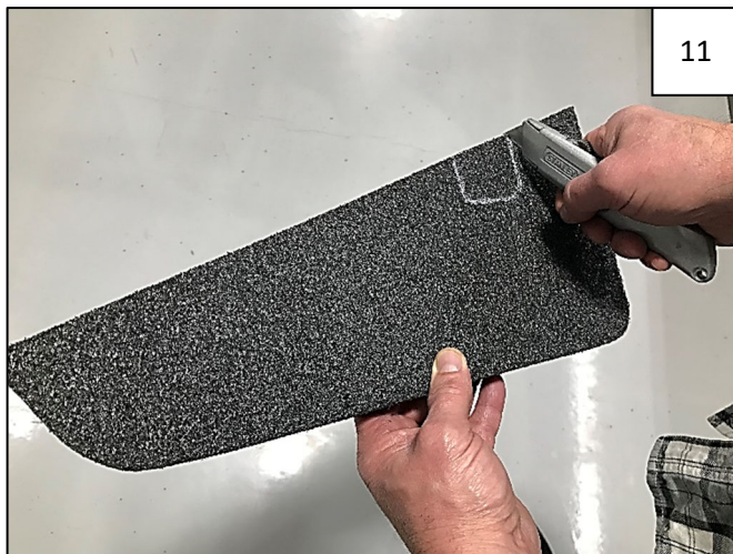
Use a utility knife to carefully cut the corresponding section out of each Foam Divider.
