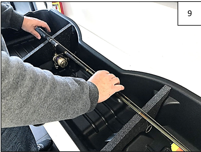
If you want to store long items lengthwise in the Underseat Storage Box, lay the item in the Box (over the top of the dividers) in the position you would like to store it in. Alternately, you may remove the dividers and skip the next steps, however, items may shift in transit.
