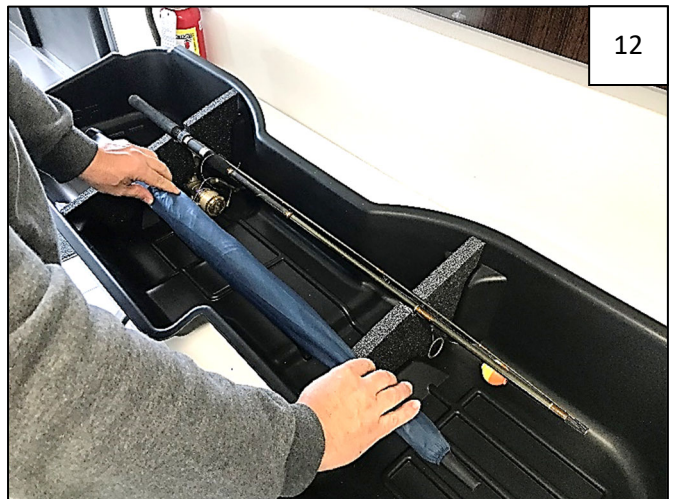
Lay long items in Underseat Storage Box as shown, pressing into the cutouts in the foam.
