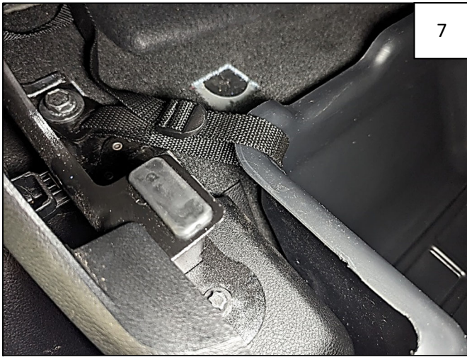
Thread buckle onto one end of safety strap. Feed other end of Safety Strap into Buckle and tighten to anchor Underseat Storage Box in place.
