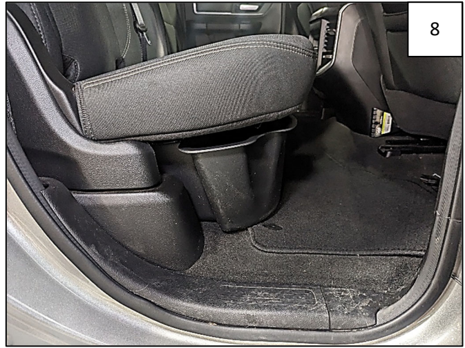
Complete Underseat Storage Box installation.
